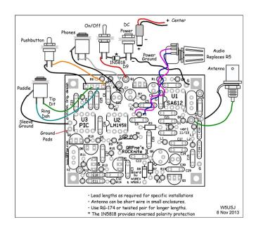
For easy frequency changing use 3-pin SIP sockets at Y1 and Y2.
